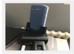
Insert the dongle into the back of the cradle, add the ethernet cable from port wall.
