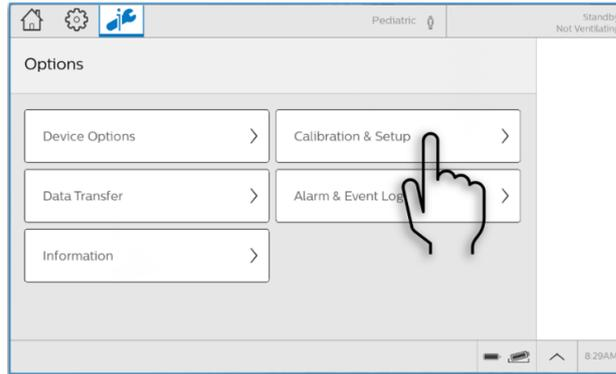
3. In the Calibration & Setup window, tap Circuit Calibration.
