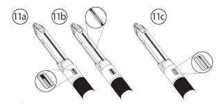
The knife can be retracted by pushing the "Reverse" button forward on the device.
