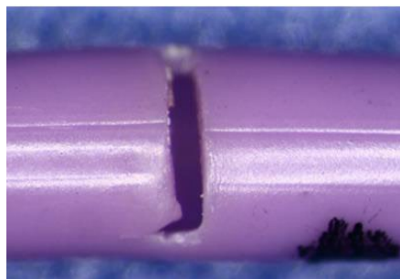
Figure 1: Example of transverse/circumferential crack in the catheter tubing
