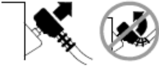
Figure 5-7 Disconnecting Defibrillation Cable from Test Post
